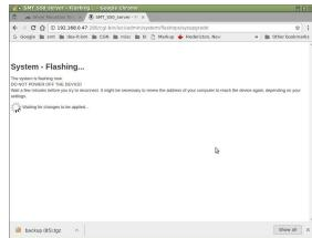
Click "Proceed" and wait several minutes. Note that the "System - Flashing...." screen will never change. It is safe to close this screen at any time. When the firmware update is completed, you will be able to access the ordinary web page, which will now have the new firmware but with all user data gone. Restore your user data:
